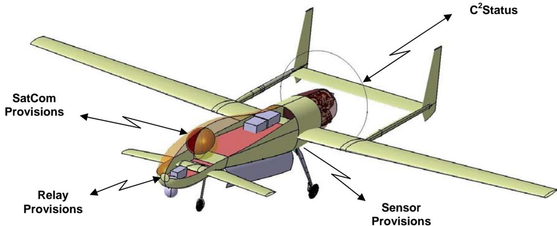
Each equipped *Mongoose*, alone or teamed, can facilitate/integrate in a net-centric, worldwide communications/command/control system, and facilitate searches.
